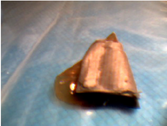
Fig. 2. A burnout sample of PEM.
